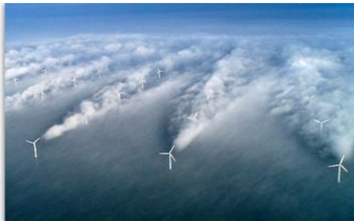
The above photograph shows the turbulence field behind the Horns Rev 1 offshore wind turbines. http://www.windturbinesyndrome.com/2011/wind-turbine-turbulence-what-are-the-micro-climate-effects/
