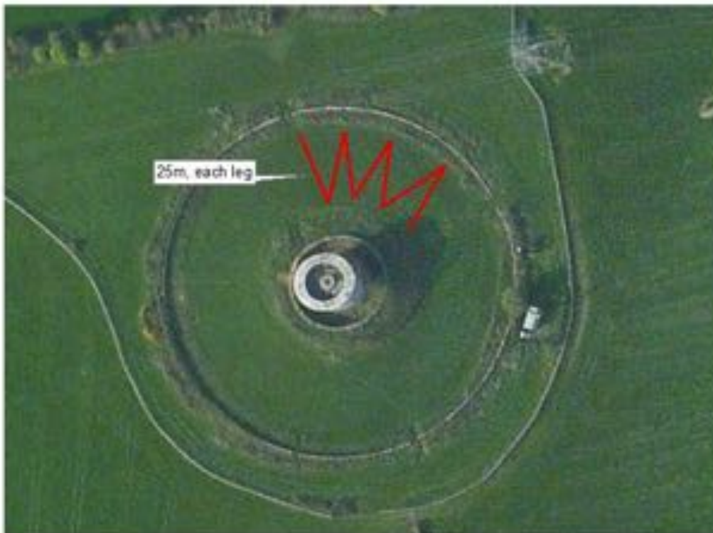
Location 3A: Each leg is 25m with 10m sample intervals – Sampled Friday, 16 th January 2015
