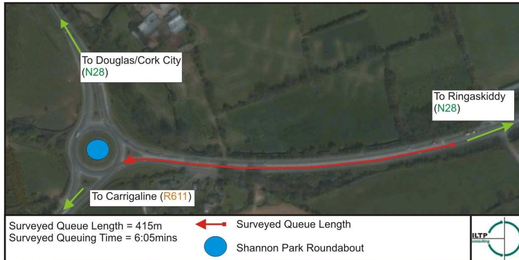
Figure 2.2 : Queuing Surveyed Westbound on N28 At Shannon Park Roundabout in PM Peak
